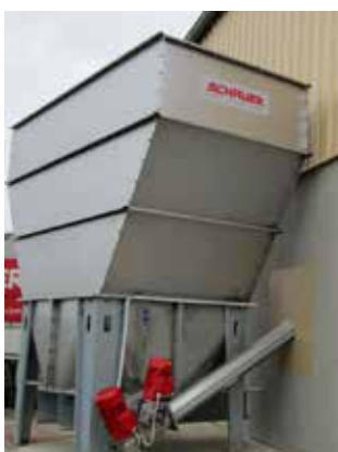
Tender-CCM storage tank made of stainless steel, up to 8 m 3 of storage volume
