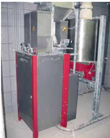
Tender-CCM storage tank made of stainless steel, up to 8 m 3 of storage volume
